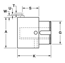
**NOTE:** The Actuating Pin Assembly is a simple pin which is forced out radially from the main body when overload occurs. When using this option, it is important to note that the housing (F bore) or external mounting hub end of the unit is the power source or input end. This part of the unit must continue to rotate for the extended pin to contact a customer supplied limit switch for shutdown or warning.
